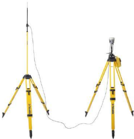
Receiver with a remote radio antenna
