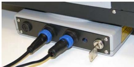
*Trimble FX with power switch key inserted and cables connected*
