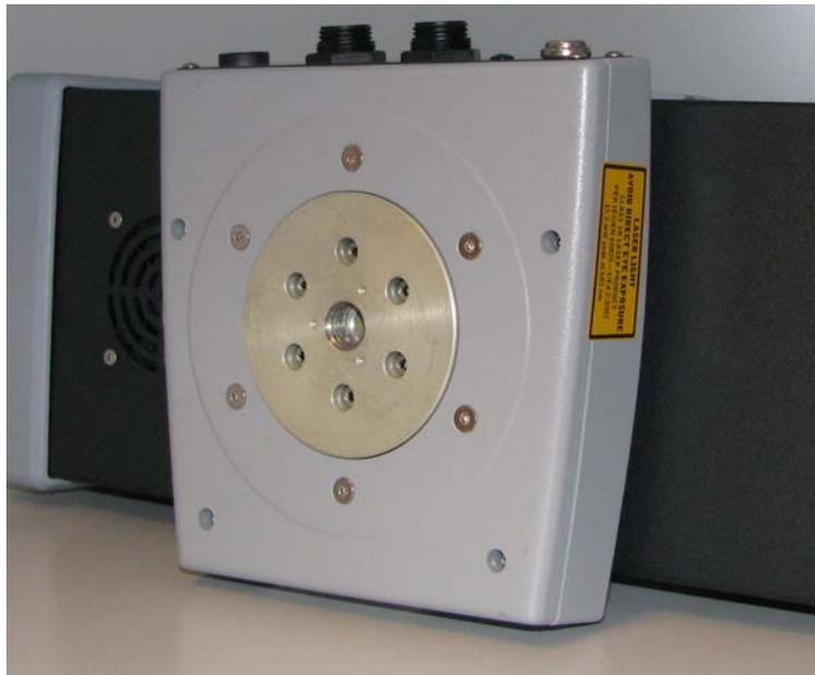
*Tripod 5/8" (survey adapter) screw hole on scanner bottom*
