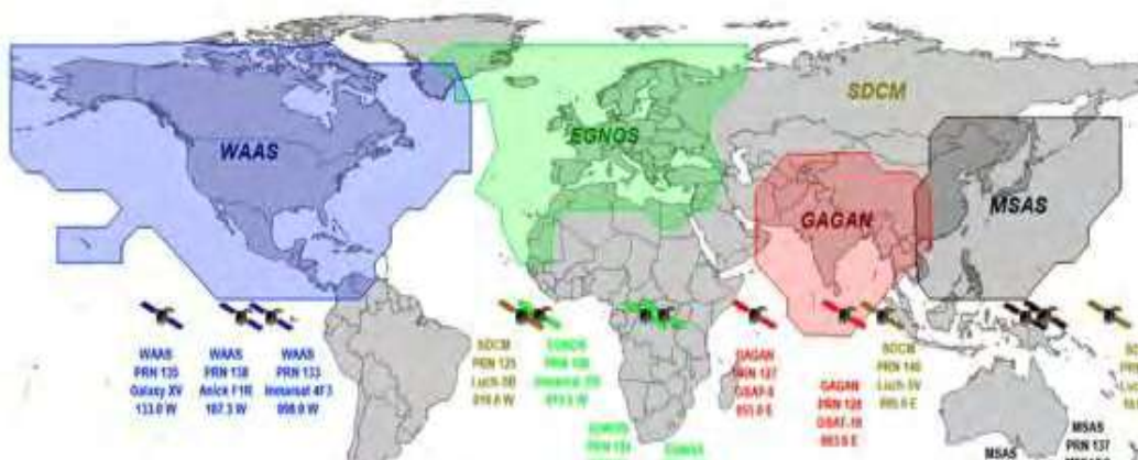
SBAS DGPS Differential correction service areas
