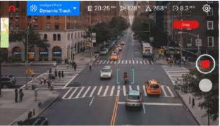
• Set the height and distance of the tracking target. The default tracking distance will be about 10ft (3m). At this time, you can also adjust the setting through the remote control. For best results while tracking, the system will keep a distance 10-40ft (3-12m) between the aircraft and target.
