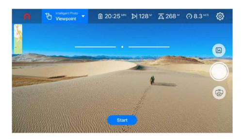
• The aircraft will fly towards the selected target and will try to avoid obstacles. During the flight you can tap other points on the screen to change the flight direction. To change the flight speed, you can adjust the speed bar in the lower center of the screen.
