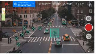
• A 3 second countdown will start automatically. After the aircraft successfully starts the tracking, the target will be surrounded by a green rectangle.
