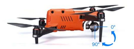
The gimbal angle can be adjusted using one of 2 methods. The camera gimbal will rotate accordingly as shown in the following figure.
