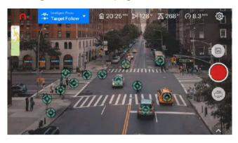
• Set the height, distance, and direction with the tracking target. At this time you can also make adjustments from the remote control. To ensure the best tracking results, please set a distance of 3-12m between the aircraft and the target.
