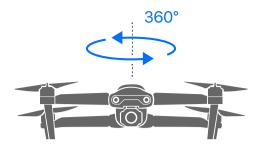
3 Hold the aircraft vertically with the nose facing downward and rotate it until the rear LED indicators on the aircraft turn solid green, indicating that the calibration is successful.
