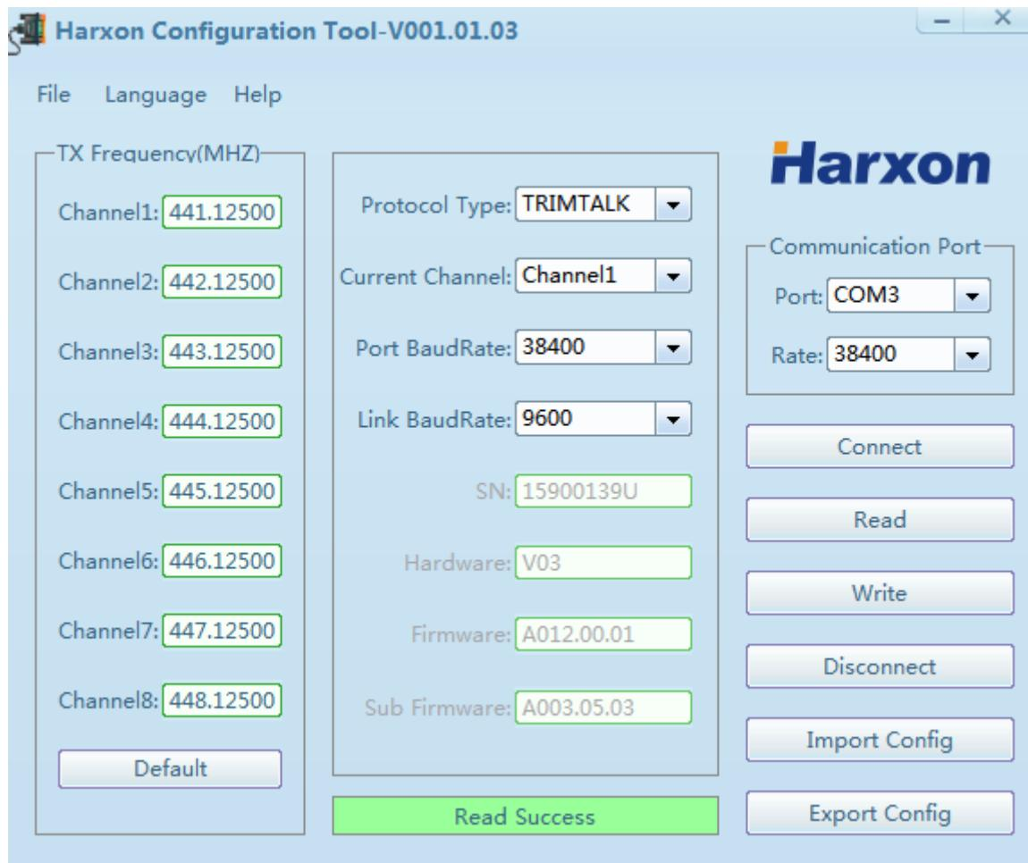
Noted: Before Configuring Radio Parameters, click “Read” **Read** Button, First read all the configuration parameters of the machine, and then make the appropriate parameter modification;
