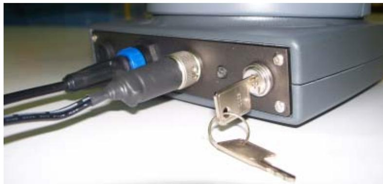
*Trimble FX power switch key inserted, cables connected*
