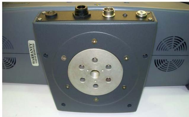
*Tripod 5/8" (survey adapter) screw hole on scanner bottom*
