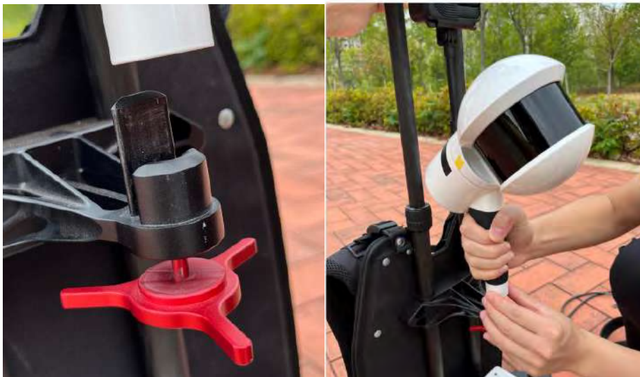
Figure 2-9 Hold the bottom to the top insert and tighten the screws
