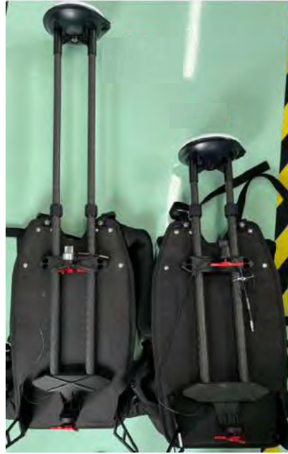
Figure 2-8 Fully withdraw the telescopic rod and tighten it
