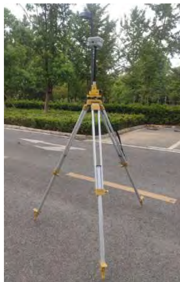
Figure 4-1 Base station erection
