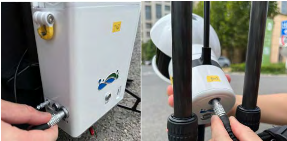
Figure 2-11 Connect the power cable (MAIN port).
