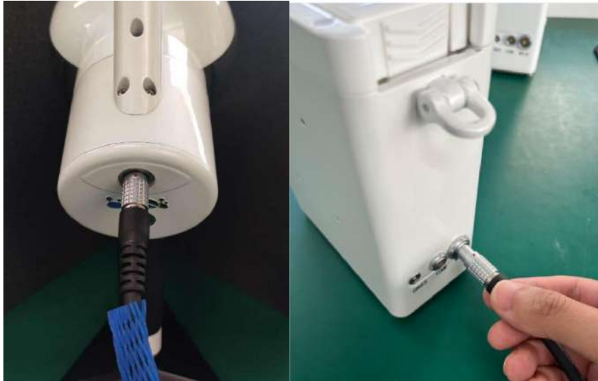
Figure 2-2 The host power cable is connected to the handheld device console and the battery compartment (MAIN port)
