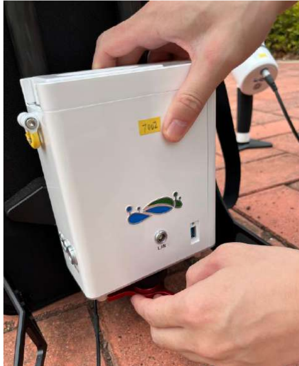
Figure 2-6 Align the battery compartment with the bottom screw and tighten
