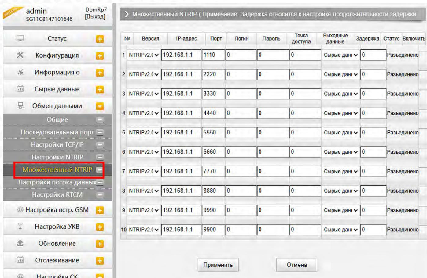
The screenshot shows the configuration interface for multiple NTRIP servers. The left sidebar contains navigation options, with "Множественный NTRIP" highlighted in red. The main area displays a table of 10 NTRIPv2 server configurations.
