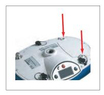
Keeping one hand on the battery still in its compartment, put the ProMark 800 the right way up. The battery will then easily slide out of the battery compartment.
