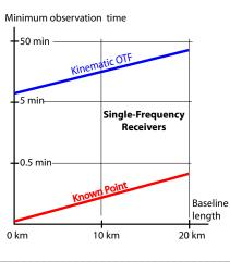
Not surprisingly, the minimum observation times in postprocessed surveys are roughly equal to the TTFF's in real-time surveys, for the same type of equipment, baseline and initialization methods.
