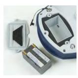
The battery used in the ProMark 800 is a 7.4-V DC - 4600 mAh rechargeable battery. It is a standard model used in many camcorders.
