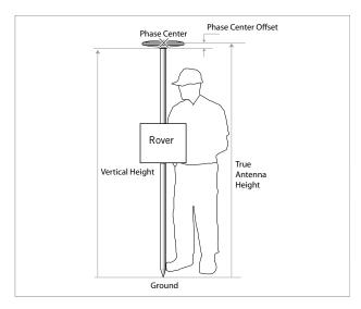
The real height of the antenna is therefore the sum of the vertical height and the phase center offset.
