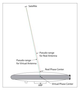
The receiver has to correct the collected data (most notably pseudo-ranges) so that they appear as if they had been collected –for each frequency– at the virtual phase center, not at the real phase center.
