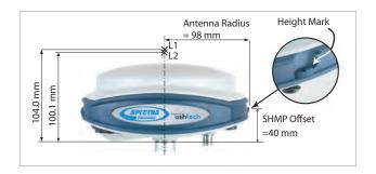
The height mark allows you to hook the measure tape onto it so you can unroll the tape down to the survey mark and read the slant height measurement directly on the tape.
