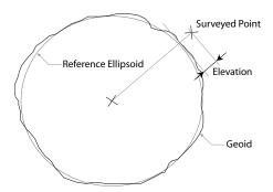
This surface is irregular depending on the density and distribution of materials on the surface of the Earth, which means the geoid may not exactly follow the natural features on the Earth's surface. (The geoid is a fictitious surface that can't be seen).
