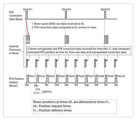
The time when position is requested is t0 and the time when the rover starts providing the position for time t0 is t1. Times t0a, t0e and t0j in the base and the rover are synchronous because they originate from the same clock which is the GNSS time.
