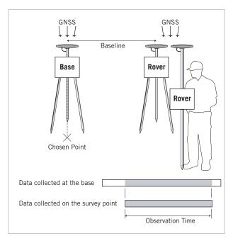
1. Two systems are used: one (the base) is operated on a chosen point while the other (the rover) is used in the working area for the survey.
