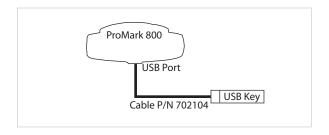
Generally speaking, after connecting a USB key to the receiver, the USB logo will appear on the screen after a while. Then three different screens (or less, depending on the content of the USB key) will be shown in succession, at a rate of 10 seconds, provided no button is pressed in the meantime. These three possible screens are shown below.
