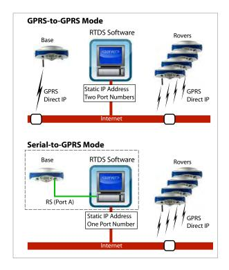
In Serial-to-GPRS mode, the base and the computer running RTDS are at the same location since a conventional RS232 serial line is used to connect one to the other.
