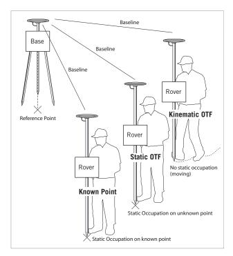
**Kinematic OTF.** For both post-processing and RTK real-time, this method does not make initialization faster but is the less constraining method in the field (although it does not release you from being careful on the operating conditions). Kinematic OTF should be used by default when there is no reference in the working area that can help secure the initialization.
