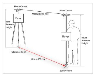
To compute the position of the mark instead of the antenna, it is necessary to instruct the rover to perform an *antenna reduction*. In an antenna reduction, the antenna heights are taken into account when computing the rover position.
